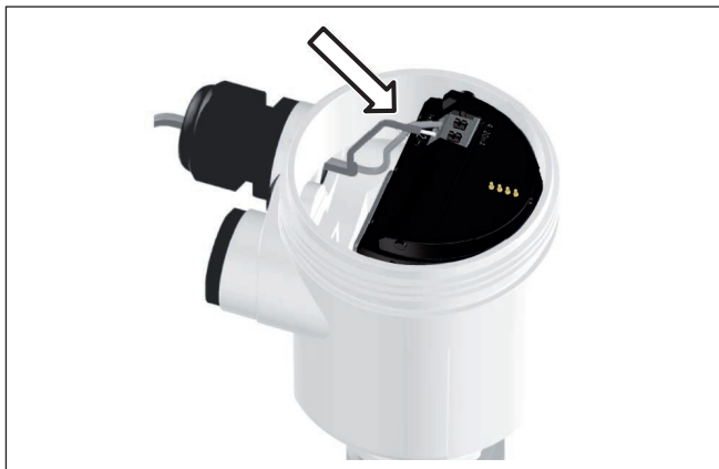
Fig. 18: Connection steps 5 and 6 - Single chamber housing
