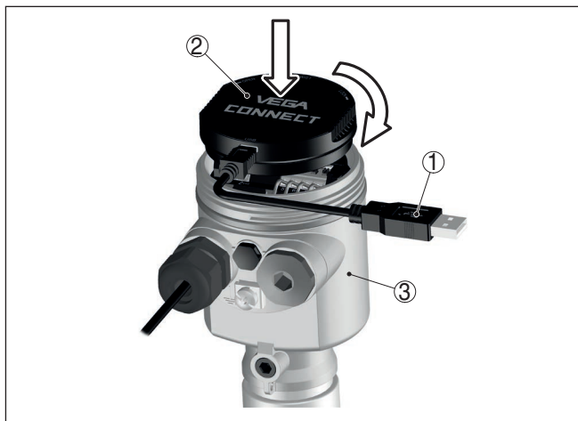
Fig. 29: Connection of the PC directly to the sensor via the interface adapter
