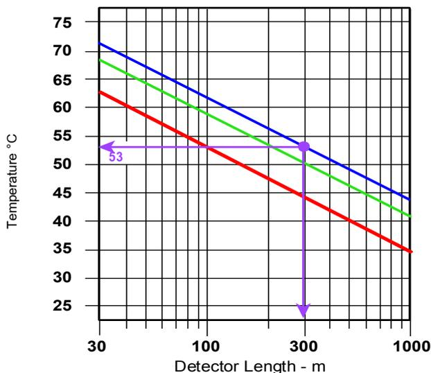
Zone Monitors are equipped with sensitivity / trip adjustments. The graphs show three typical settings; 3V, 2V and 1V..
