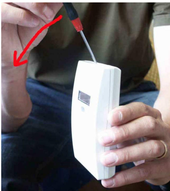
Figure 3 Closed housing seen from the side The housing is opened by inserting a screw driver and pushing left (to the front side). The locking hooks will then be released.
