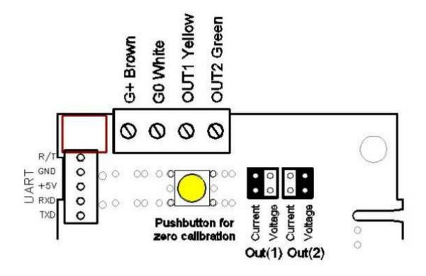
Figure 1. Terminals and jumpers on CF8-D/W-IN. The darker positions are default settings. The push button is for forcing a manual zero point calibration if the sensor does not enter the automatic zero calibration mode just by flowing zero gas.
