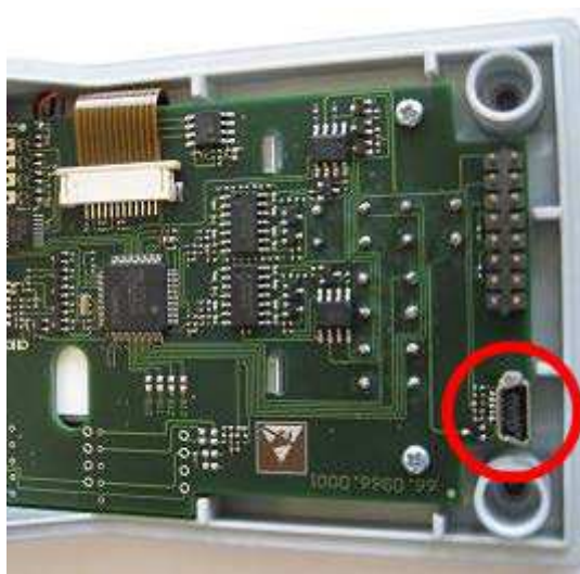
Figure 11: Location of the service port on the top side of the circuit board
