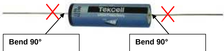
Figure 14: Shortening and bending the connections
