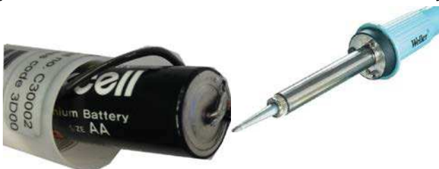
Figure 13: Unsoldering the battery
