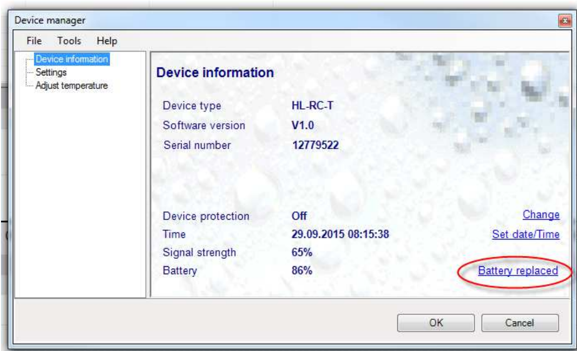
Figure 16: Setting the time after a battery change
