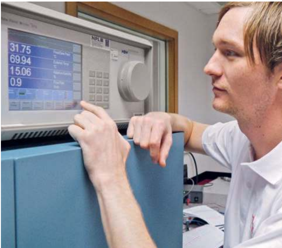
Chris Aicken, laboratory manager, Rotronic UK at a MBW dew point mirror.
