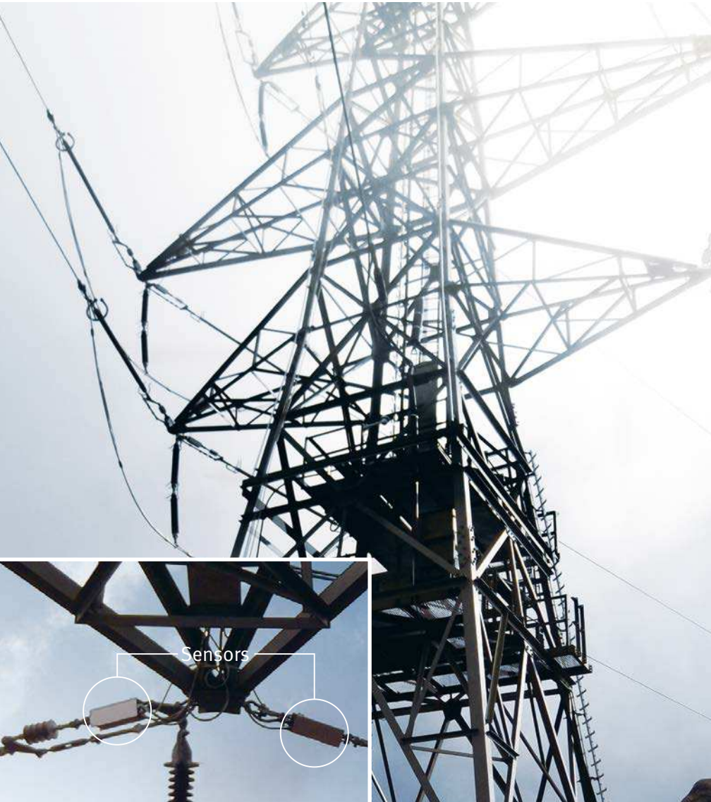
The ice load is measured at especially critical points by strain gauge sensors attached to the masts
