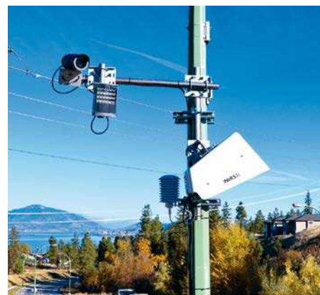
Network of Road Weather Information Systems (RWIS) in Kelowna BC with ROTRONIC HC2-S3-L, installed by CSC.
