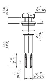
Housing (standard temperature range –40 °C ... +100 °C), M12 x 1, IP 67
