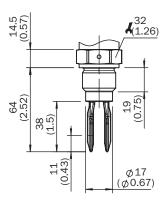
Housing (enhanced temperature range –40  $^{\circ}\text{C}$  ... +150  $^{\circ}\text{C}$ ), DIN 43650 incl. plug angled, IP 65
