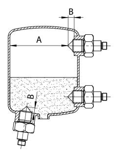
Installation in a pipe for dry running protection. A ≥ 40 mm (1.57)
