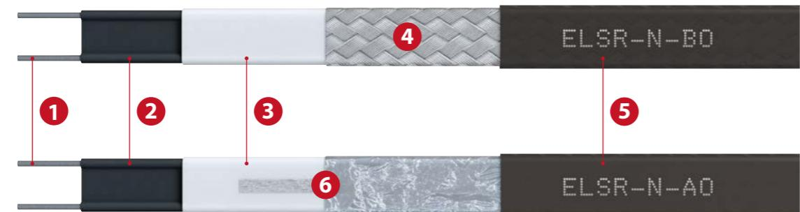
**1 Bus wire** Nickel plated copper**2 Self-regulating heating element****3 Insulation****4 Protection** Protective braid (Cu, tin plated)**5 Outer jacket****6 Protective conductor connection** see 4 or Cu, tin plated with aluminium foil
