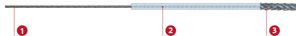
**1 Heating conductor** Stranded or coiled
