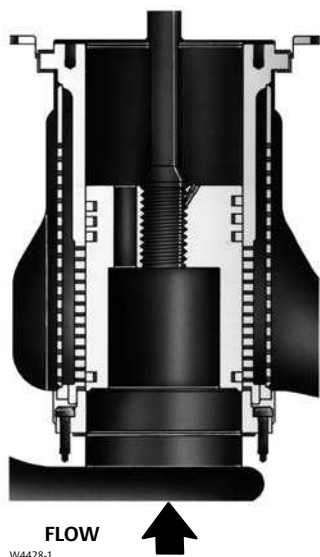
Figure 11. Fisher EHD Trim with Whisper Trim III Level D Cage (NPS 8 through 14 Globe Valves)
