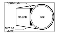
Over time temporary coupling compounds (e.g. Petroleum Gel) may gradually sag away from the sensor resulting in reduced signal strength and finally complete loss of signal. Warm temperatures, moisture and vibration will accelerate this process. Dow Corning Silicone Compound #4 as supplied with the UF D5000 (and available from Micronics Limited) is recommended for semi-permanent installations.
