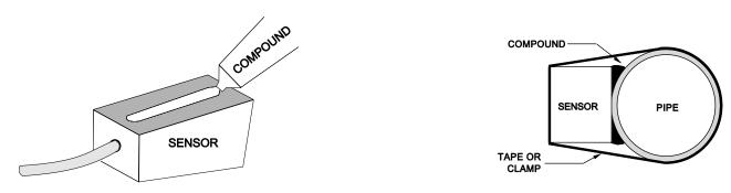
For proper operation the transducer must be fixed securely to the pipe with coupling material between the transducer face and the pipe. Sensor installation with excessive coupling compound or use of epoxy can result in gaps or voids in the coupling and cause errors or loss of signal. Insufficient coupling compound will create similar conditions.
