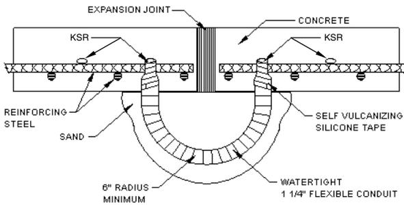
8. Attach cable with nylon tie straps on approximately 12" centers such that installed cable will be between 2" and 3" below the snow melting surface of the concrete.
