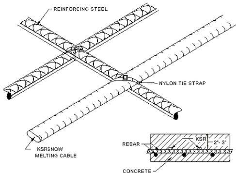
**DO NOT** Use metal wire to secure heating cable to rebar or steel mesh - electrical hazard and short circuits could result!
