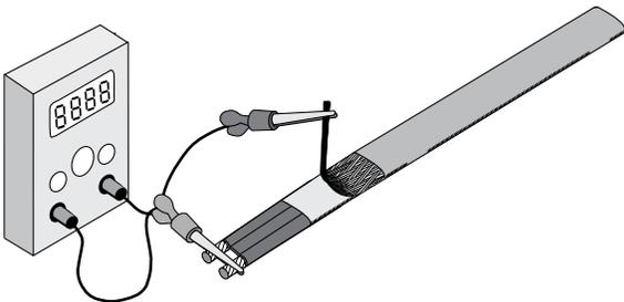
Connect the positive lead of the megger to the cable bus wires and the negative lead to the metallic braid.
