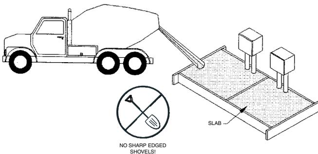
**IMPORTANT:** During the pour, care should be taken to minimize the chance of cutting or damaging the heating cable, causing short circuits.
