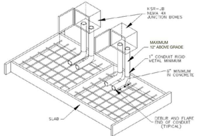
4. Route heater cable ends through rigid galvanized conduit into power/end termination box and temporarily fix both ends of the cable in the box. Leave at least 6” for terminations later.
