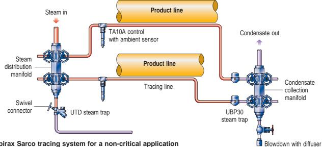
Spirax Sarco tracing system for a non-critical application
