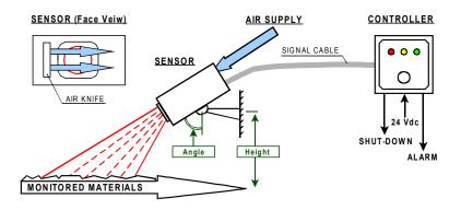
The sensor is located above or beside the materials transit path (conveyor, roadway, etc.) by means of the adjustable mounting bracket and aligned such that the monitored hazard passes through the sensor's field of view. The distance and angle of the sensor determine the width of the monitored path.
