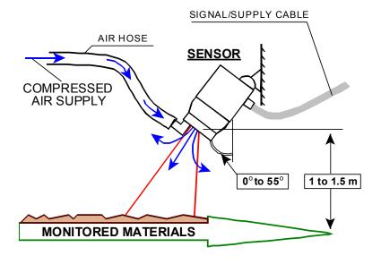
The table below shows the width of the monitored product at the Lowest and Highest sensitivity settings. This is based on the sensor being installed at a 45° angle.
