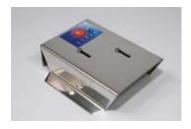
The Floodline Point Sensor is a compact sensor for vertical or horizontal mounting. Water touching its stainless steel probes activates the alarm. Used with the stainless steel Floodline Guard Plate to give heavy duty physical protection and assist fixing and adjustment.
