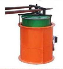
Top, bottom or side flanges may be used to attach handling equipment, if preferred to manual lifting. A range of dedicated products is available but many standard forms of handling device are suitable.
