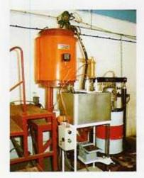
Complete access to the drum while heating enables pumps and stirrers to be employed. The drum and heater can be integrated into the system, often eliminating the first process vessel, and continuous feeding of material, at regulated temperature and flow rate, can easily be achieved.
