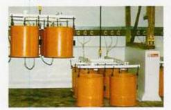
capacity of an oven. For example, one particular award winning installation of 3 THERMOSAFE units heats 20 drums per day. The ease at which capacity can be adjusted, to meet varying throughput demands and the varying heating requirements of different materials, is in stark contrast to the fixed facility of an oven.
