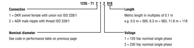
Example: 1 m heated hose, 4 mm nominal diameter, 230 V supply voltage, AGR connection
