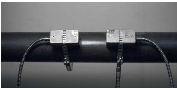
Illustration 4: Sensor mounting with tension straps and clamps
