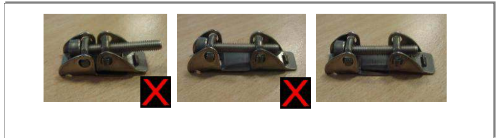
Illustration 14: Clip arrangement for correct tensioning
