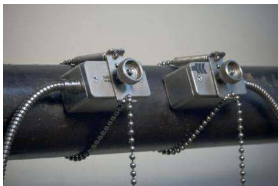
Illustration 7: Sensor mounting with clips and chains
