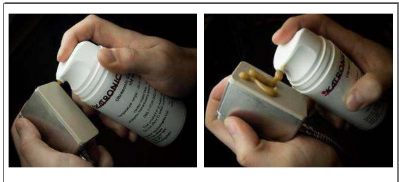
Illustration 5: Application of acoustic coupling gel
