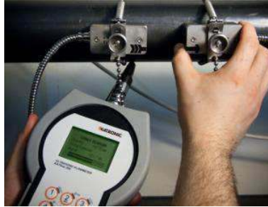
Illustration 6: Correct positioning of the sensors
