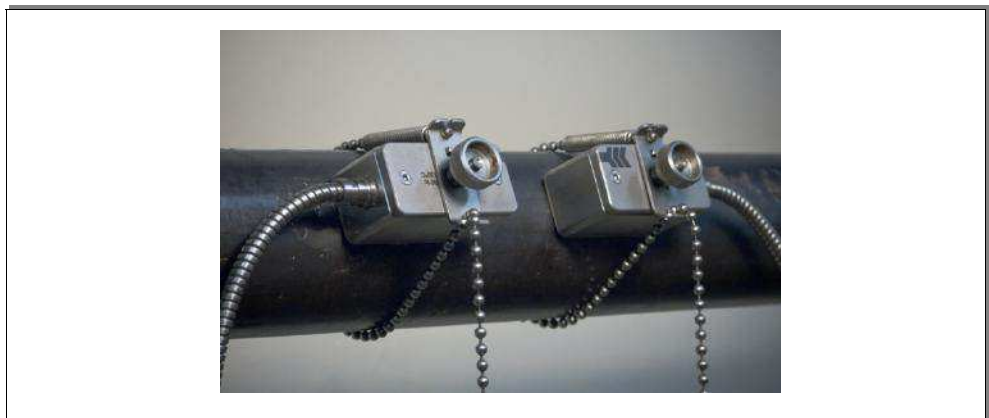
Illustration 7: Sensor mounting with clips and chains
