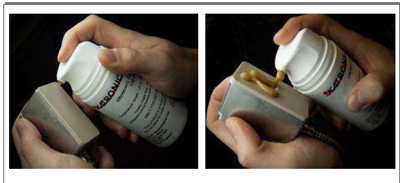
Illustration 5: Application of acoustic coupling gel
