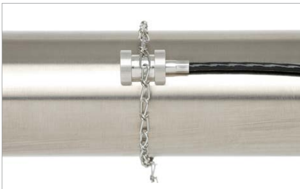
PT100 transducer fixed to pipe
