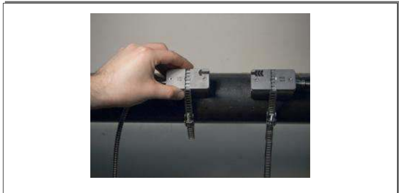
Illustration 6: Correct positioning of the sensors
