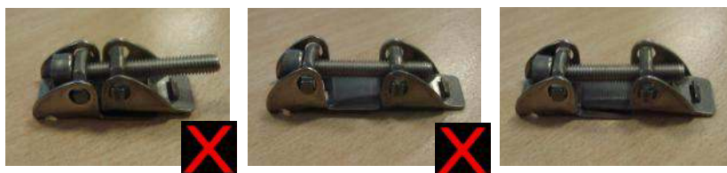
Illustration 9: Clip arrangement for correct tensioning
