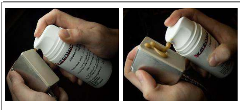
Illustration 5: Application of acoustic coupling gel
