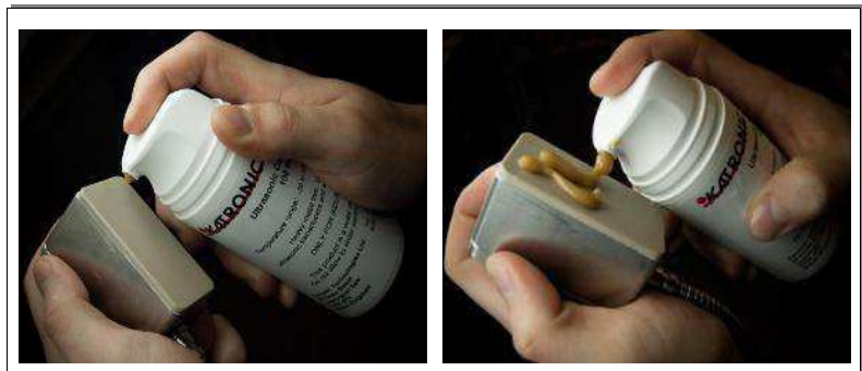
Illustration 7: Application of acoustic coupling gel
