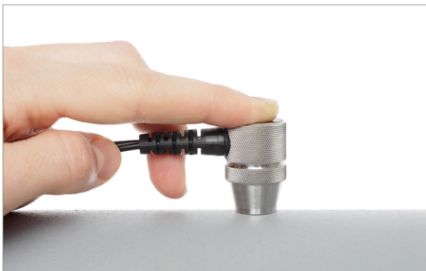
Wall thickness gauge NT in use
