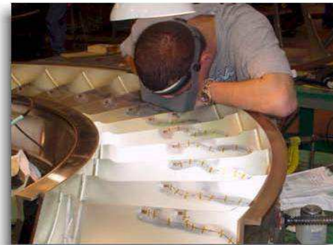
Strain Gage Instrumentation of a large fan by AEI.
