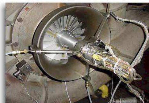
Aerodyn slip ring performing strain survey on compressor. Pictured is a 36 contact slip ring capable of 90,000 RPM. A similarly designed 72 contact slip ring was provided to Williams International for fan and compressor strain surveys on the FJX/TSX and EJ22 turboshaft engines at speeds to 75,000 RPM.
