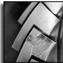
Detail of strain gage attachment on compressor blade
