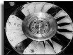
Detail of strain gage attachment on compressor blade
