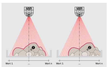
Particularly determining the center of gravity increases system availability:
