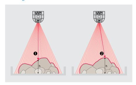
In addition to volume and throughput, the Bulkscan® LMS511 also calculates the height profile of the bulk materials. This way large rocks can be detected in a timely manner before blocking or damaging equipment in downline machining processes.
