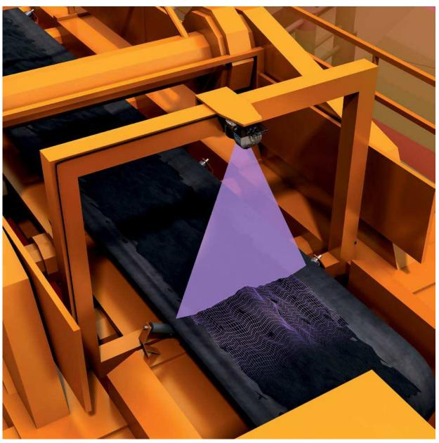
A laser scanner emits a pulsed-laser beam. When it hits the bulk material, it is reflected and registered in the scanner receiver. The time it takes for the pulse to be emitted and received is directly proportional to the distance between scanner and bulk materials.
