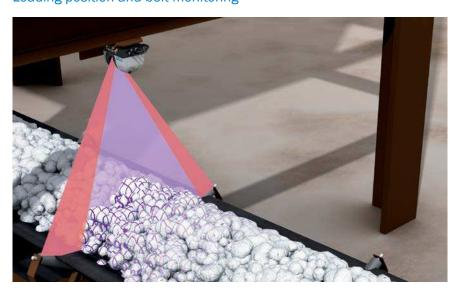
Shifting of the conveyor belts can sooner or later lead to belt wear. Bulkscan® LMS511 detects the loading position and limit at an early stage using the belt monitoring function. This ensures optimal system utilization.
