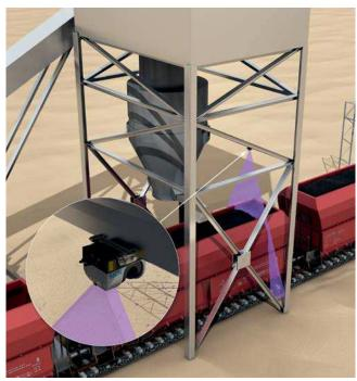
The non-contact measuring Bulkscan<sup>®</sup> LMS511 detects the profile of the bulk material on the conveyor belt. The flow rate is calculated using the belt speed and the bulk material profile. This makes it possible to create a feedback control system that provides optimal belt speed and ensures economic belt utilization.
