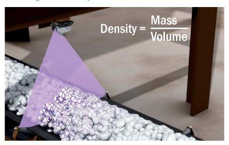
Calculating the material density makes it possible to assess the condition and quality of the material. The bulk density can be calculated in real time in combination with a belt scale.
