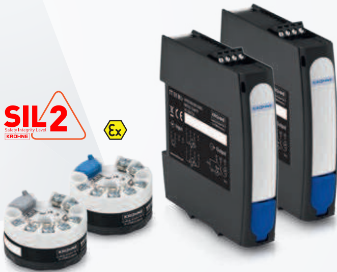
OPTITEMP TT 51 C, TT 51 C Ex OPTITEMP TT 51 R, TT 51 R Ex Highly precise, universal, programmable 2-wire HART® transmitters for thermocouples and resistance sensors with current output, full assessment on SIL2 according to IEC 61508:2010
