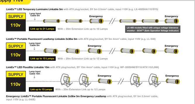
The above are example typical configurations, please contact us for confirmation of maximum linkable light chains for specific requirements in terms of cable extensions and the use of different lights.
