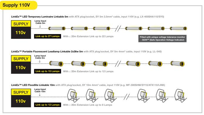
The above are example typical configurations, please contact us for confirmation of maximum linkable light chains for specific requirements in terms of cable extensions and the use of different lights.
