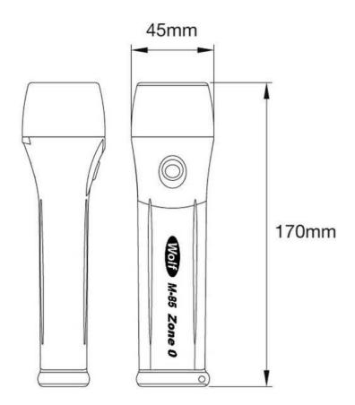
210 lumens LED Spot Beam (approx  $7^{\circ}$ ) with a Wide Angle Fringe Beam (approx  $55^{\circ}$ )
