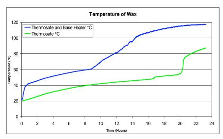
Temperature of Wax measured at hardest to heat location (base of drum in centre)
