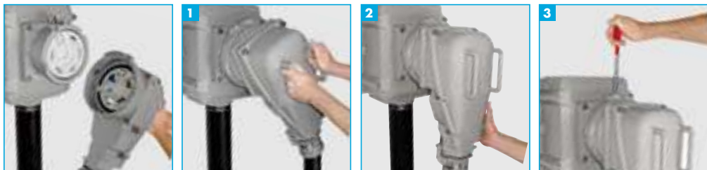
1 Off load engagement. 2 Automatically watertight. 3 Locking the plug in the socket closes the pilots and connects the main circuit.
