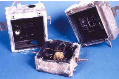
SX and BPG Range Enclosures after BS6387 Testing
