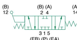
hand lever 3 position 4-way closed center w/detent
