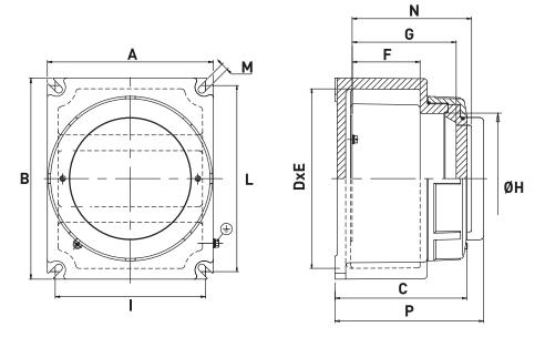
GUB../QL Series enclosures c/w internal mounting plate - Aluminium
