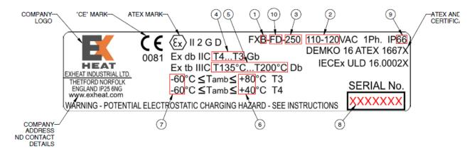
Typical nameplate when fitted with a thermostat
