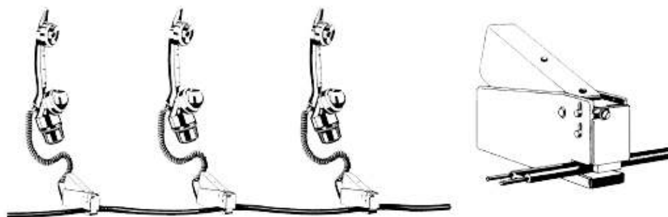
3. With fixed cable, for plug-connected handsets and/or permanently installed wall telephones
