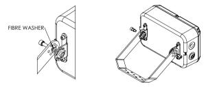
3. POSITION STIRRUP TO PREFERRED ANGLE AND SECURE USING REMAINING M6 SREW, SPRING-WASHER AND NUT (ITEM 9)
