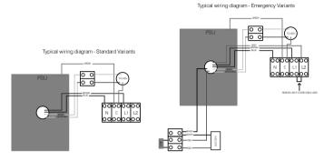
Wire the Mains cable into the terminal block. Provision has been made for this and identified as the E (Earth), L1 (Live switched), L2 (Live permanent) and N (Neutral) terminals. There are two pairs of contacts for each of these to facilitate a mains cable that can be looped in and out of the unit. The L2 terminals on a standard unit are not electrically connected but allows them to be used on the same circuits as *emergency bulkheads*.
