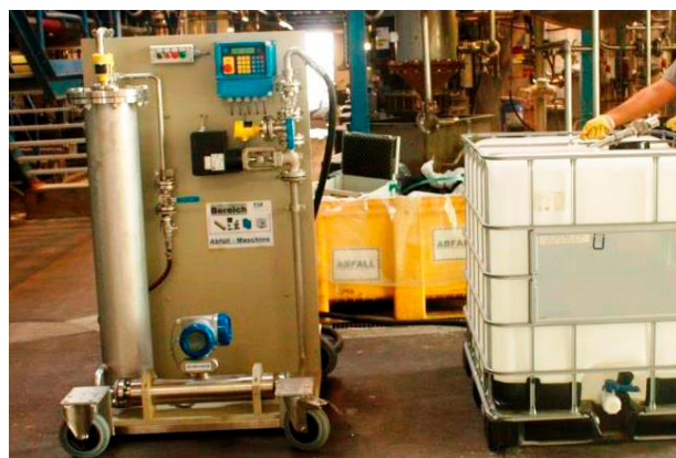
Mobile measuring system with the OPTIMASS 7300 C
