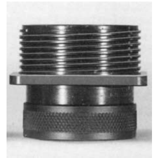
Standard double-lead Acme. Two parallel threads.
