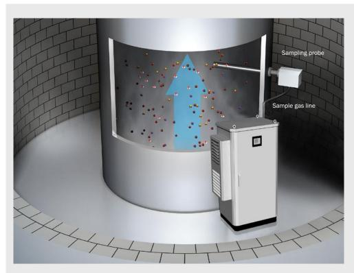
MERCEM300Z measures using hot extraction: The flue gas is extracted using a sampling probe and is transported to the analyzer via a sample gas line. All components in contact with the sample gas, such as the probe, sample gas line, and converter in the analyzer are heated above the dew point.
