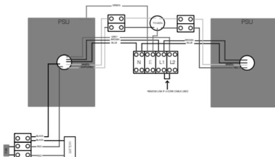
Typical wiring diagram - Emergency Variants
