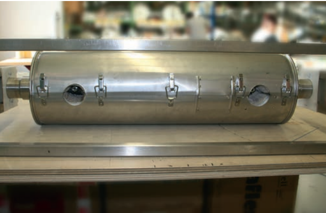
Heating jacket with sheet metal outer jacket
